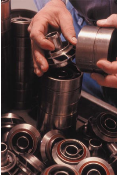
Figure 3. Multistage centrifugal pump units consist of stages with rotating impellers and stationary diffusers stacked together to meet the lift requirements for various applications.
